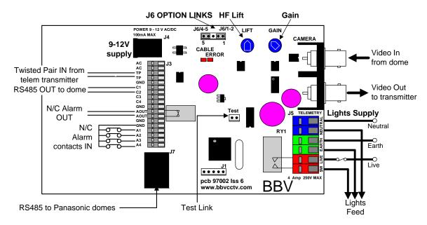
Fig. 2 Rx100 Iss6 PCB connections
